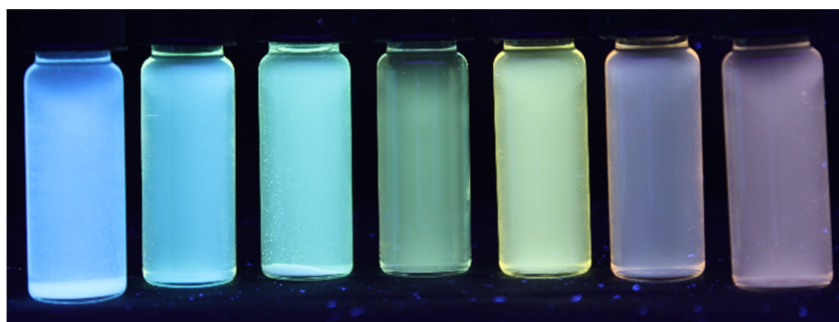
Figure 2. Fluorescence of 6p with variable solvent polarity (left to right: cyclohexane, toluene, ethyl acetate, dichloromethane, N,N -dimethylformamide, acetonitrile; \lambda_{\text{exc}} = 365 nm, hand-held UV lamp).
